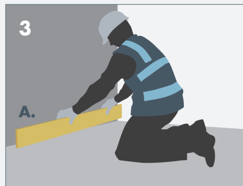
3 Place the edge strip up against the perimeter.
