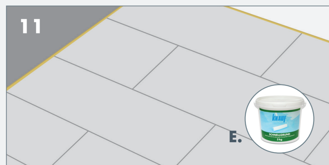
11 Once the floor is laid and clean, apply Knauf Floor Primer prior to adhering any floor finish. For vinyl floor finishes always apply a suitable self-leveller.
